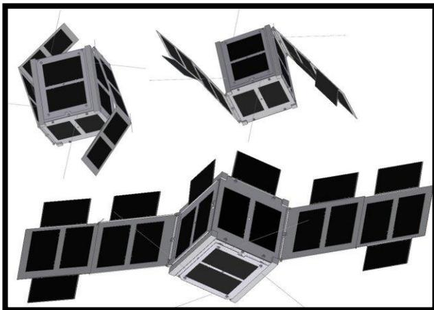
**Figure 4: Deployable CubeSat Solar Arrays**
