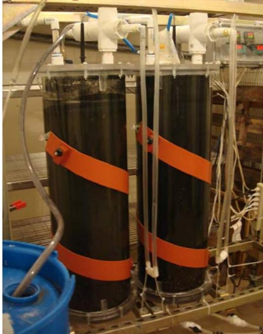
Figure 4-2. Pilot scale IBR systems (56 L each) contain temperature control, pH control, variable hydraulic retention times, and ports for easy sampling and maintenance.
