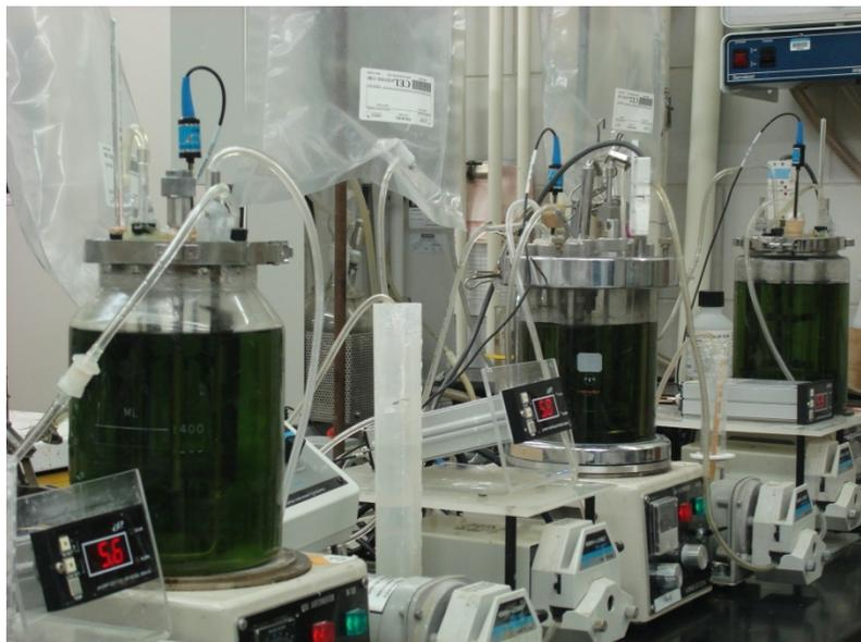
Figure 3-2. Anaerobic batch digester setup using manure and cheese whey.
