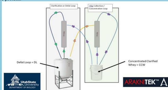
**Fig. 1** TFF system. TFF is more efficient than traditional filtration systems because it is self-cleaning and more reliable. Water and particles in it move tangential to the pores in the filter. This perpendicular flow helps to disrupt buildup of the larger particles on the filter itself. If this system is further improved, it has the potential to greatly improve the manufacturing process of synthetic spider silk proteins.
