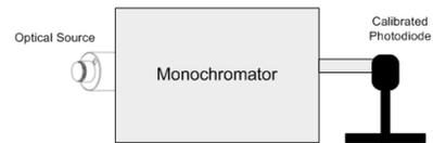
Figure 3: Instrumentation setup for characterizing the emission spectrum.
