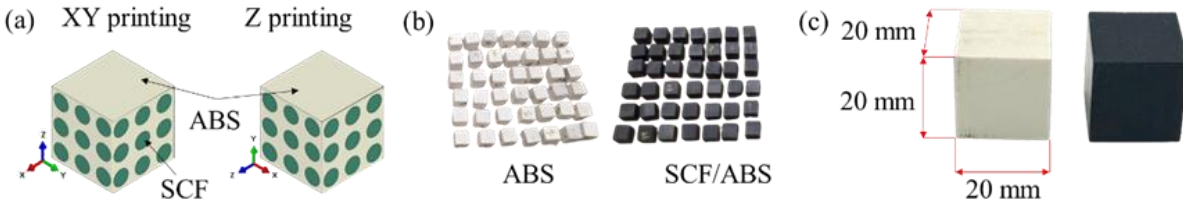
Figure 1. ABS and SCF/ABS specimens: (a) schematic of printing configuration (b) prepared specimen (c) zoomed-in view of the prepared specimen.
