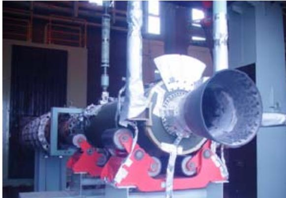
Figure 8. B0 motor after static firing test
