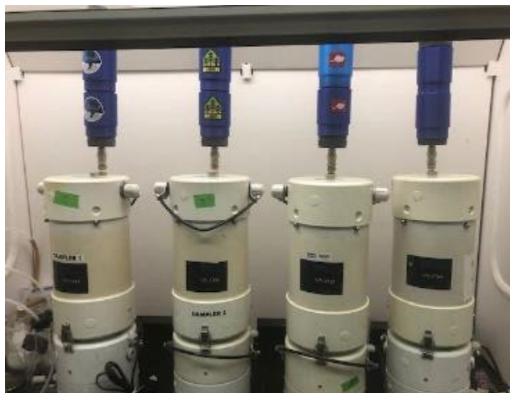
Fig. 17. PFAS air sampling assembly with Minivol active sampler
