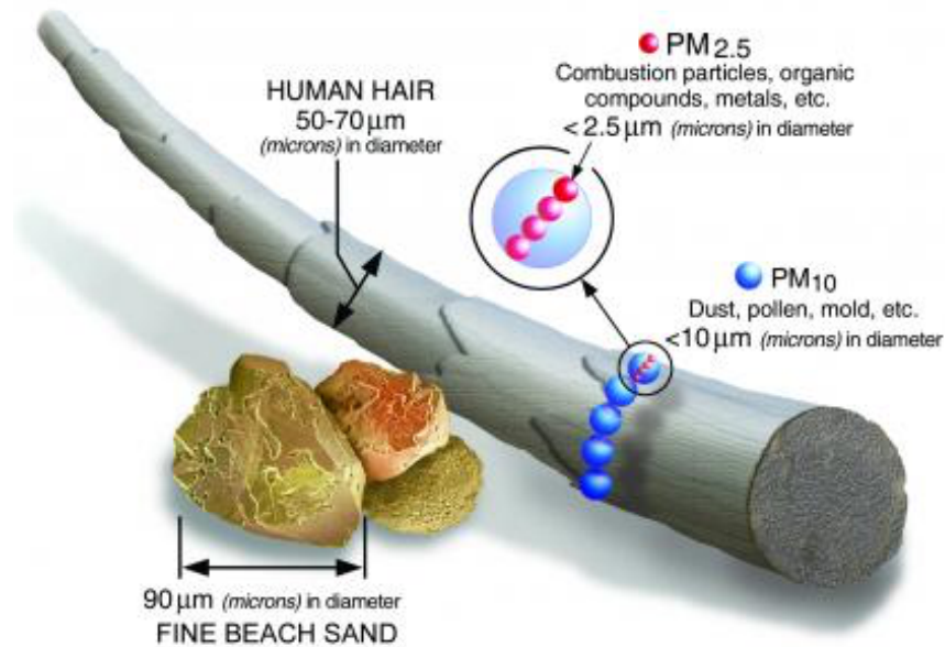
Figure 1. Particulate matter size. Particulate matter is divided into coarse ( \leq 10 \mu\text{m} ), fine ( < 2.5 \mu\text{m} ), and ultrafine ( < 0.1 \mu\text{m} ) particles. Approximately 5 \text{PM}_{10} molecules span the width of a human hair, and 4 \text{PM}_{2.5} molecules fit the diameter of one particle of \text{PM}_{10} . Image taken from the U.S. Environmental Protection Agency.
