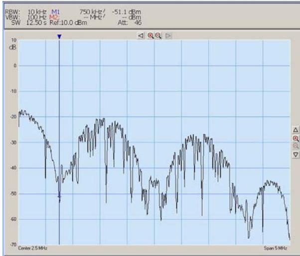
**Figure 6: Spectrum of In-Phase Demodulated Baseband Signal**
