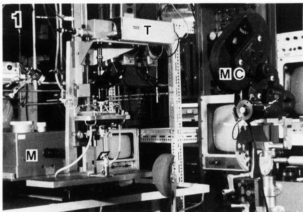
**Figure 1.** Light microscope modified for high resolution *in vivo* microscopy, using monochromatic light source (M) and television (T) imaging. MC, motion picture camera modified for recording video images.
