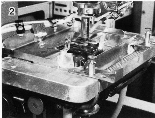
**Figure 2.** Microscope stage modified to hold small laboratory animals for *in vivo* microscopy.
