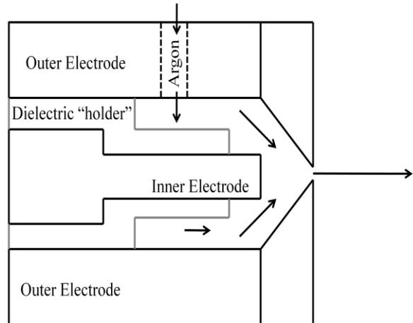
**Figure 7: Schematic of the Thruster with a Nozzle Plate On**
