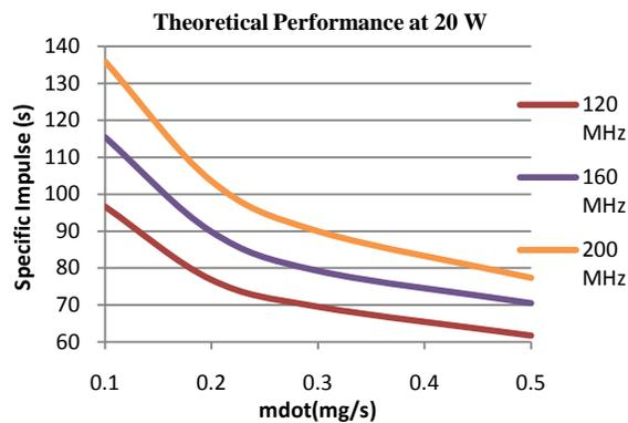
**Figure 3: Constant-Power Section of Theoretical Results**
