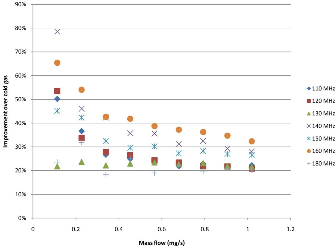
**Figure 12: Frequency Sweep Results, 40 W power, Plastic 0.025” Nozzle**
