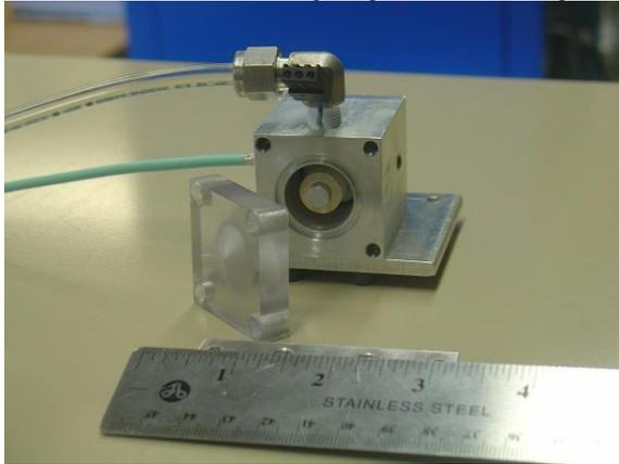
**Figure 6: Picture of RF Microthermal Thruster. A Nozzle Plate and Ruler are Shown for Scale**
