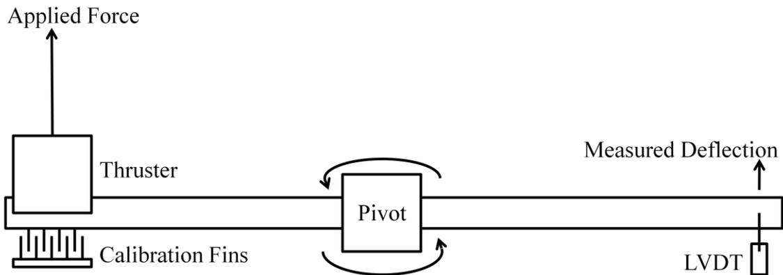
**Figure 5: Schematic of the Micronewton Thrust Stand.**
