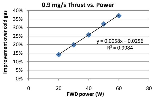
**Figure 11: Linearity of Thrust with Increasing Power**
