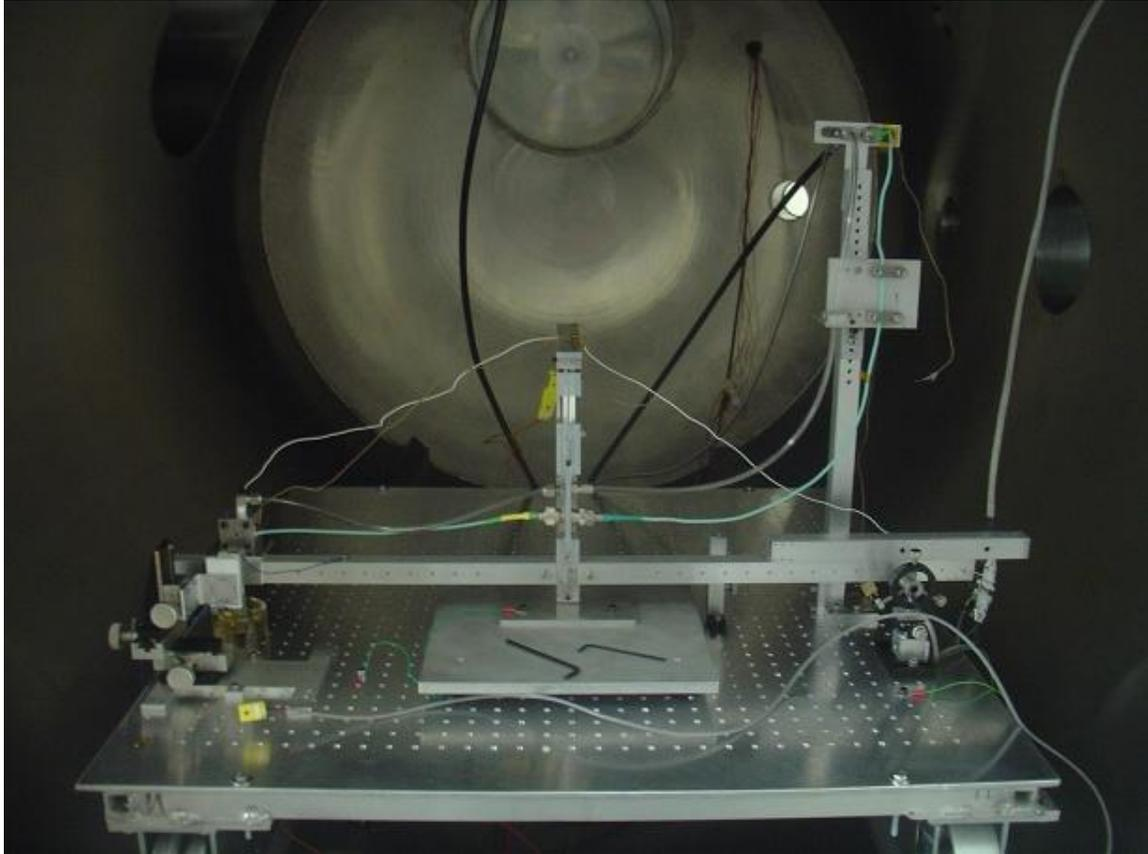
**Figure 4: Picture of the Micronewton Thrust Stand**
