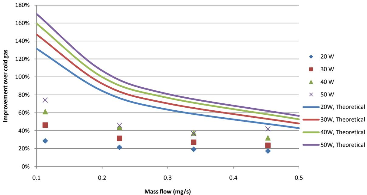
**Figure 16: Theoretical vs. Experimental Results at 140 MHz with Nozzle On.**
