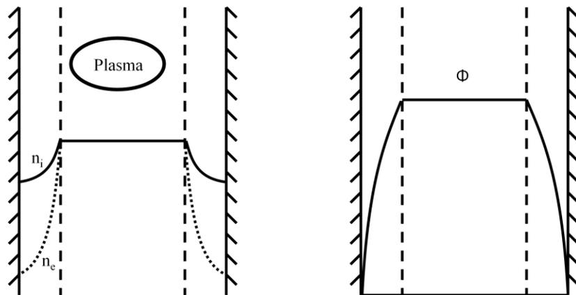
**Figure 1: Plasma sheath schematic: on the left, the ion and electron densities between two electrodes, and on the right the potential 'well' formed by the sheaths**
