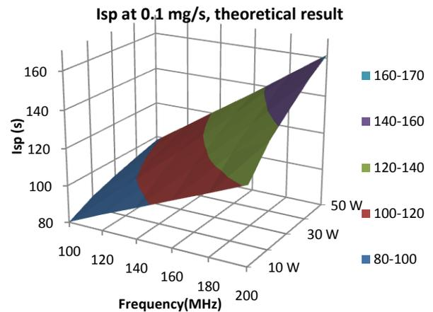
**Figure 2: A Section of the Theoretical Performance Results for the RF Microthermal Thruster**
