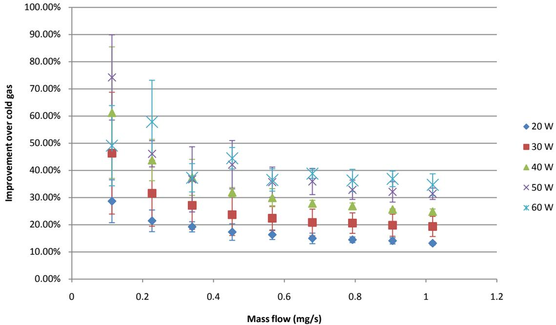
**Figure 10: Power Sweep Results, Plastic 0.025” Nozzle, 140 MHz frequency**
