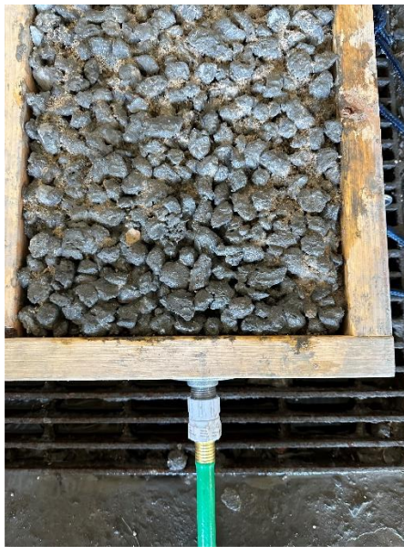
Figure 4-13: Less sand observed in area within 3-5 inches of hose attachment
