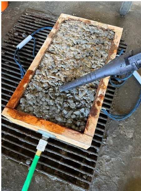
Figure 4-15: Vacuuming Model 2 during maintenance method test
