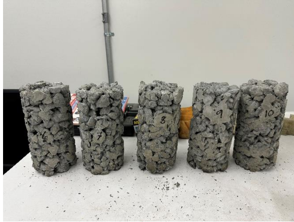
Figure 4-5: Normal cement pervious concrete cylinders
