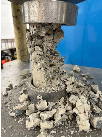
Figure 4-3: Example of 7-day compressive strength testing for rapid-set cement mix
