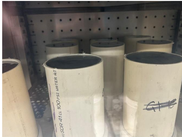
Figure 4-6: Setup of pervious concrete specimens in freeze-thaw chamber
