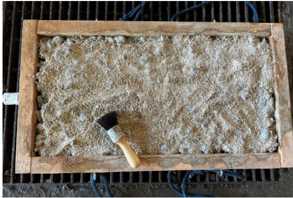
Figure 3-12: A brush was used to spread sand on each model for three tests
