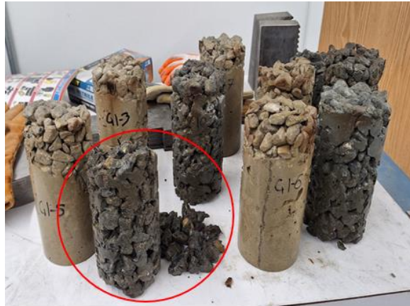
Figure 4-7: Structural deterioration of concrete after freeze-thaw testing
