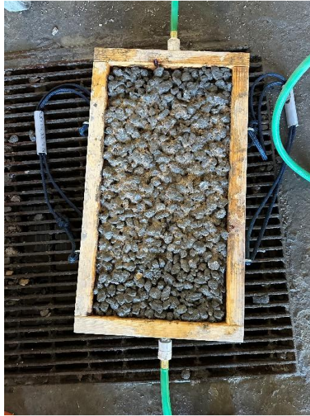
Figure 4-19: Final result of upward flush system and vacuuming for Model 3
