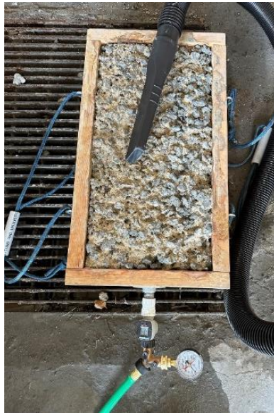
Figure 3-13: Experimental setup of model with hose attachment and vacuum
