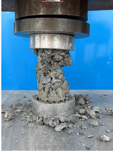
Figure 4-1: Example of 7-day compressive strength testing for normal cement mix
