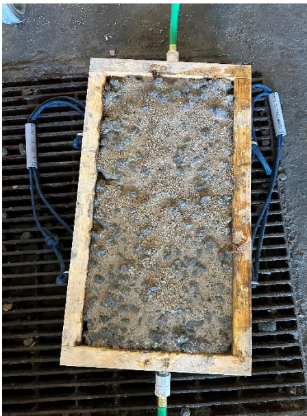
Figure 4-18: Upward flush system working in a maintenance test for Model 3
