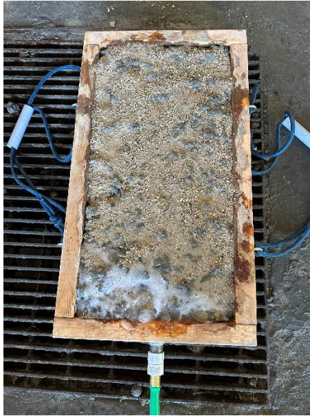
Figure 4-14: Water flowing through upward flush system attachment during test
