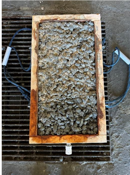
Figure 4-16: Final result of upward flush system and vacuuming for Model 2
