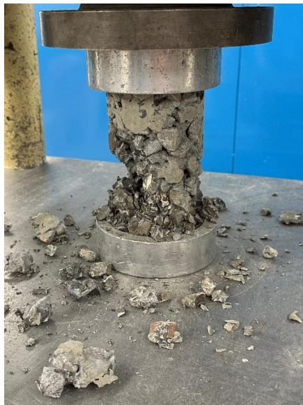
Figure 4-2: Example of 28-day compressive strength testing for normal cement mix
