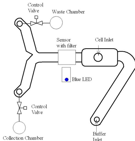
**Figure 4 Extremophile microfluidics analysis instrument diagram.**
