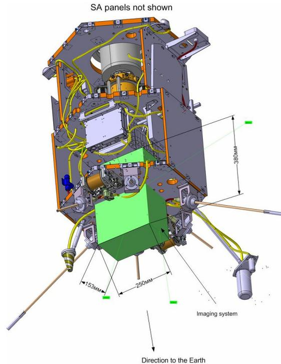
**Figure 1 UNESCOsat satellite based on the ISS-Reshetnev Yubileyniy platform. The green box is the available payload area.**
