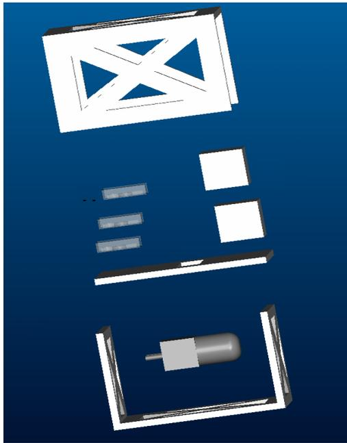
**Figure 3 Exploded view of Shawenella experiment showing outer structure, growth chambers, vessels, electronics support plate, pump and bottom structure.**
