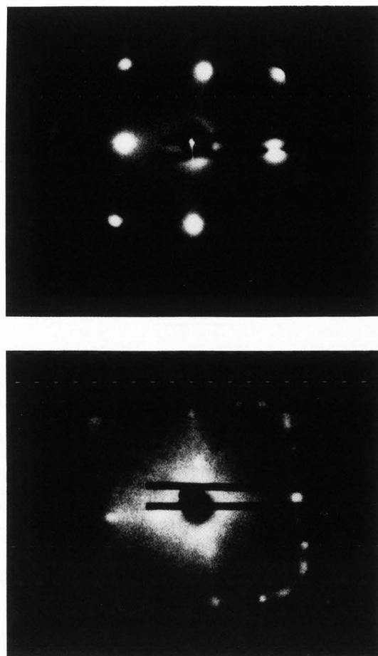
Figure 1. LEED patterns of Hg overlayers of Ag(100). The top pattern shows the p(1x1) structure (identical to the substrate) that occurs following an exposure of 6 langmuirs ( $6 \times 10^{-6}$  torr seconds) of Hg to Ag(100) at 87 K. This corresponds to the deposition of two monolayers of Hg on Ag(100). The bottom LEED pattern shows the p(1x4) overlayer formed by depositing five monolayers of Hg on Ag(100) at 87 K (15 langmuirs exposure).
