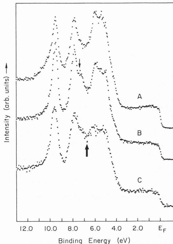
Figure 6. The EDC's of one monolayer of Hg on Ag(100) following adsorption at 30 K (A), after annealing the surface to above the Hg overlayer melting transition (B) and reannealing the surface, and above the Hg overlayer melting transition (C). Note the appearance of a new feature after annealing (little arrow) and the change in the density of states between the Hg 5d bands and Ag 5d bands. (M. Onellion, J. L. Erskine, and P. A. Dowben).
