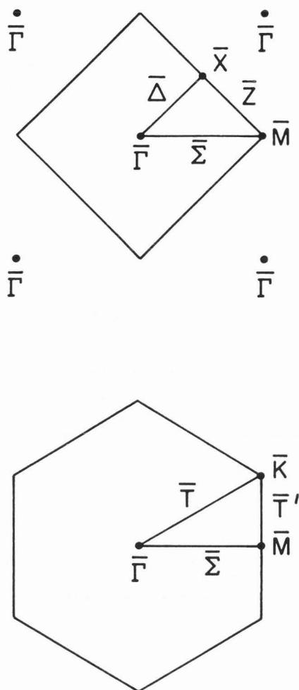
Figure 3. The high symmetry points and lines of the surface Brillouin zones of a  $C_{4v}$  or four fold symmetric surface (top) and a  $C_{6v}$  or six fold symmetric surface (bottom).
