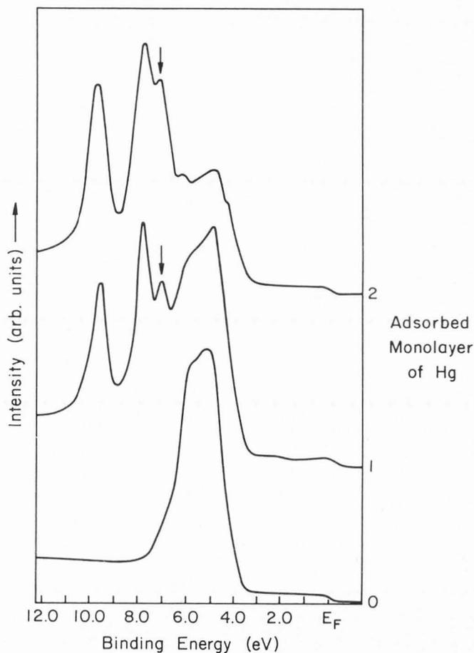
Figure 5. EDC's of the clean Ag(100) surface and following the deposition of one and two monolayers of Hg on Ag(100) at 87 K. For all spectra the photoelectrons are collected normal to the surface and the vector potential of the incident light is parallel to the surface and along  $\bar{\Gamma}-\bar{X}$ . The photon energy is 50 eV. The "split off" Hg  $5d_{5/2}$  like orbital is indicated by an arrow.
