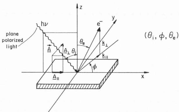
Figure 2. The geometry of angle resolved photoemission indicating incidence angle  $\theta_i$ , electron emission angle  $\theta_e$ , and orientation angle of the electron wave vector with respect to the crystal  $\phi$ . As is indicated in the figure the vector potential of the incident light has a perpendicular component and parallel component with respect to the surface as does the electron wave vector.
