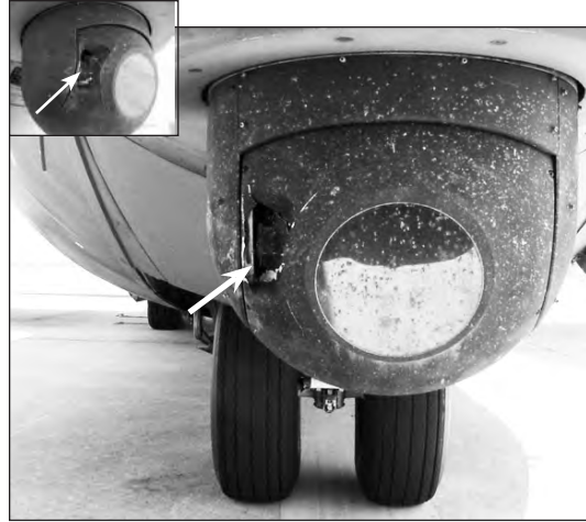
Figure 1. Damage to the AN/AAQ-17 Infrared Detecting Set on an MC-130H aircraft resulting from a strike with a Lesser dawn bat ( Eonycteris spelaea ) in Thailand. (Photo courtesy Major T. R. Murphy, Chief of Flight Safety, 353rd Special Operations Unit, U.S. Air Force)
