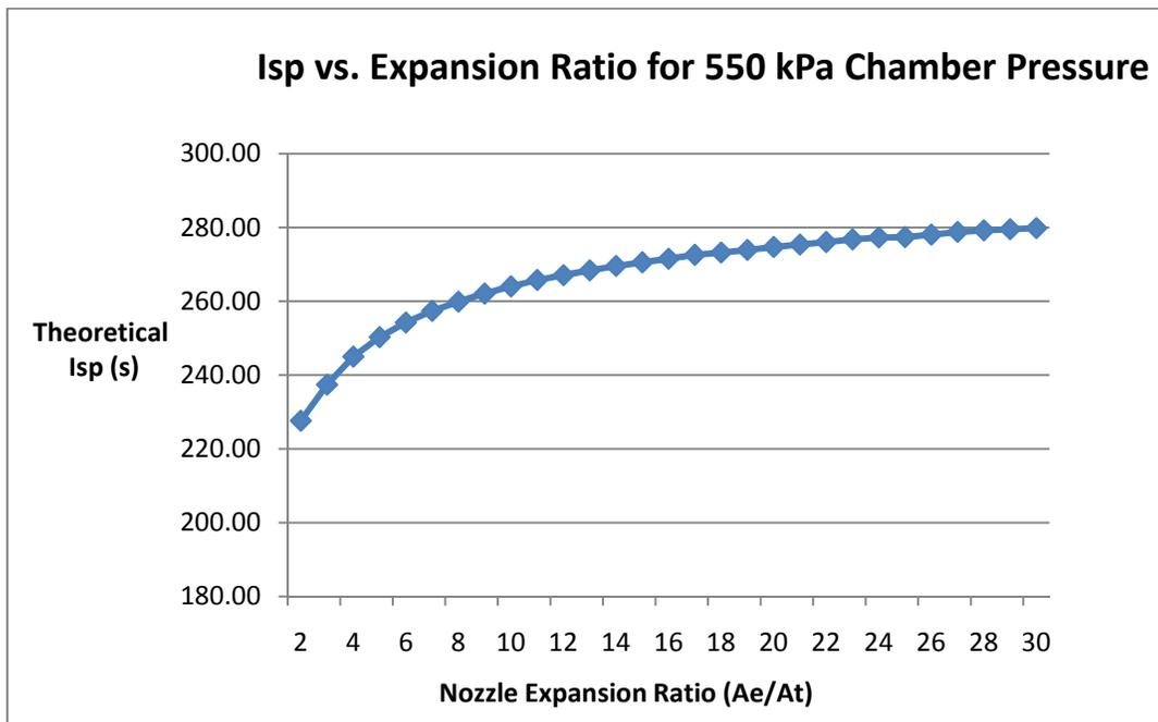
Figure 2. Plot of theoretical  $I_{sp}$  vs. Nozzle Expansion Ratio for a chamber pressure of 550 kPa.
