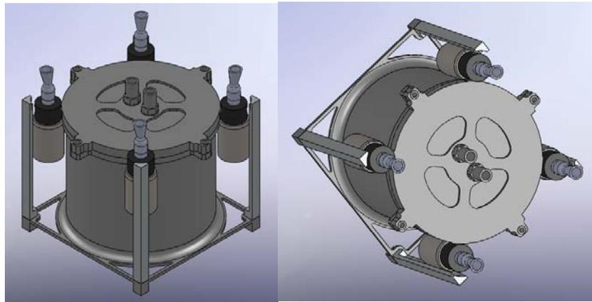
Figure 6. Cylindrical tank with vertically mounted thruster prototype Micropropulsion system assembly.
