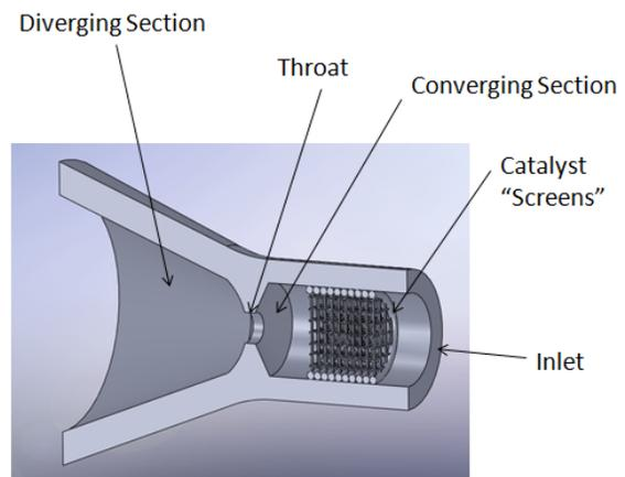
Figure 3. Prototype catalyst (left) with nozzle and chamber section view (right).
