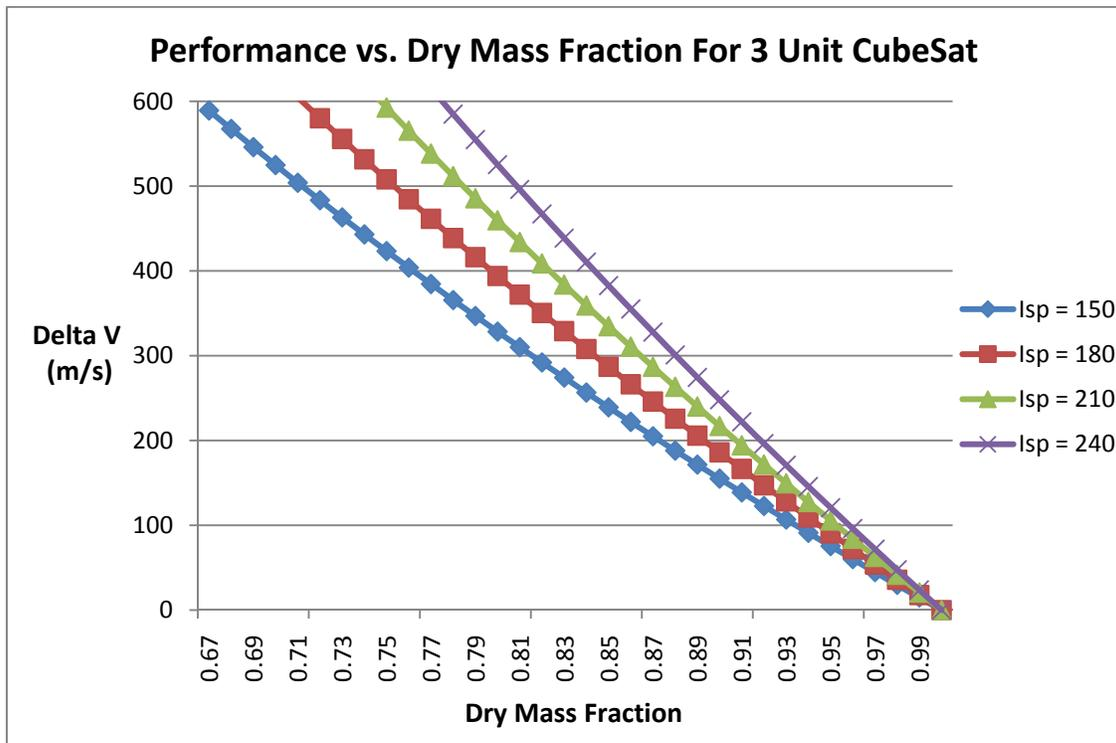
Figure 1. Performance vs. Dry Mass Fraction for various  $I_{sp}$  values.
