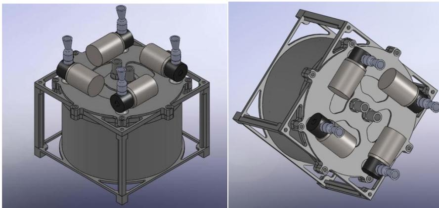
Figure 5. Cylindrical tank and cap prototype micropropulsion system assembly.
