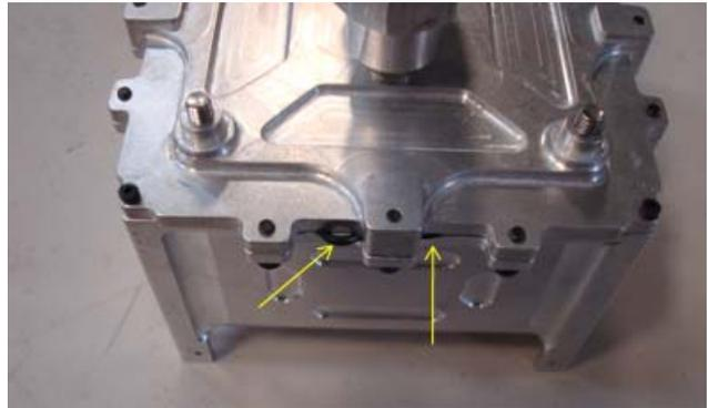
Figure 7. O-ring shown protruding out of the tank and cap.
