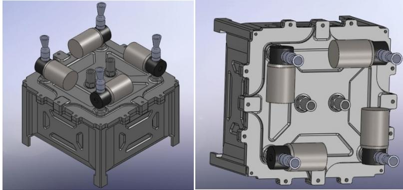
Figure 4. Cubic tank and cap prototype micropropulsion system assembly.
