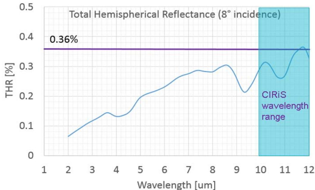
NIST measurements of a CIRiS carbon nanotube source shows reflectance  $< 0.36\%$ , resulting in emissivity  $> 0.996$
