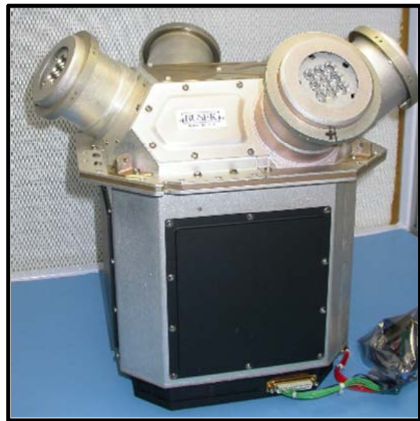
Figure 2: NASA ST7 Cluster of 4 independently operated colloid thrusters with 90 days' propellant supply, 4 power processing units (PPU), field emission cathode, and digital control and interface unit (DCIU)
