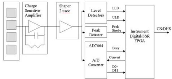
**Figure 4 Schematic of STEIN Signal Processing Chain for Each of the Four Detector Pixels.**
