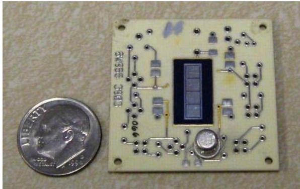
**Figure 1 Silicon Semiconductor Detector, Showing the 1 x 4 Pixel Array**
