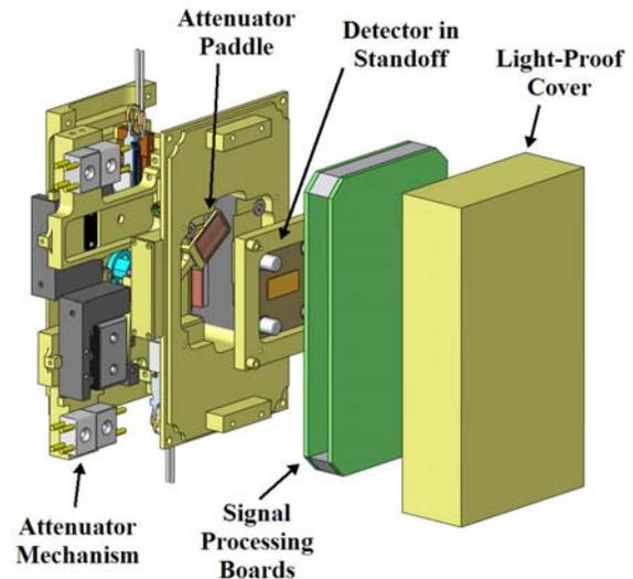
**Figure 8 STEIN Exploded View, Showing Arrangement of Detector and Signal Processing Boards**
