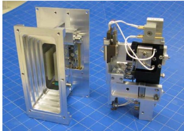
**Figure 9 Housing and Detector (Left), Attenuator Mechanism (Right)**
