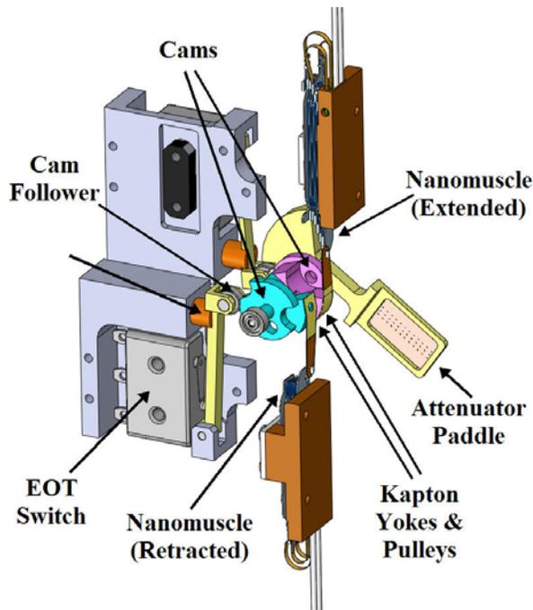
**Figure 6 STEIN Attenuator Mechanism in the Open Paddle Position**
