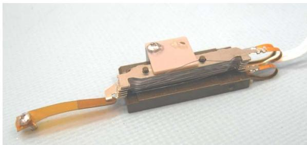
**Figure 7 NanoMuscle (Retracted) on Vespel® Base with Kapton® Yoke**
