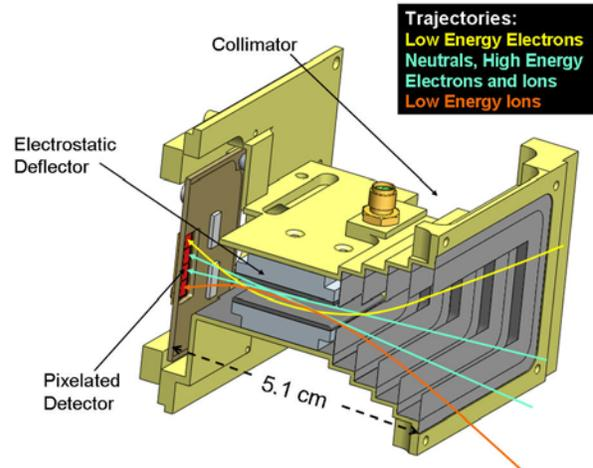
**Figure 2 Cutaway View of STEIN Showing Electrostatic Deflection (Attenuator Not Shown)**
