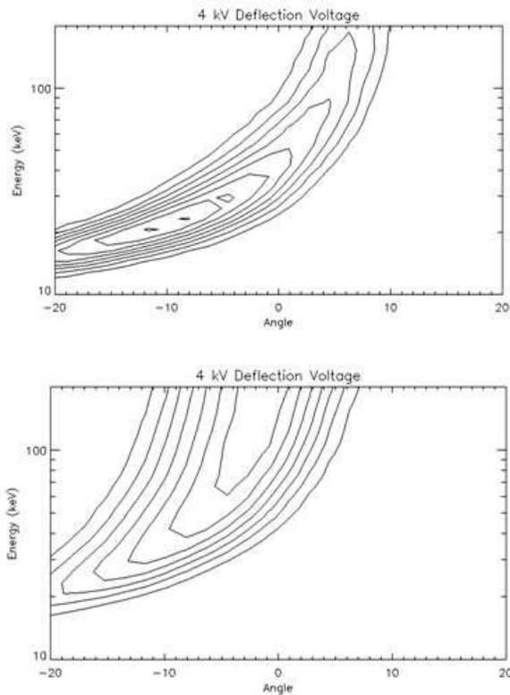
**Figure 3 Simulated Response to Charged Particles at the Maximum Deflection Voltage for an Edge Pixel (Top) and a Center Pixel (Bottom).**
