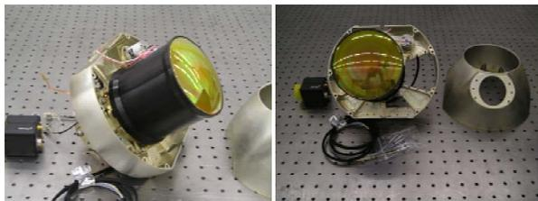
**Figure 6: UAV dual-FOV telescope mounted to the ball gimbal bulkhead**
