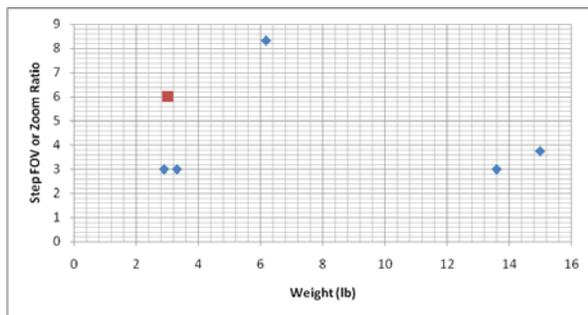
**Figure 4: Zoom ratio or FOV step ratio versus lens weight of various LWIR dual-FOV and zoom lenses**
