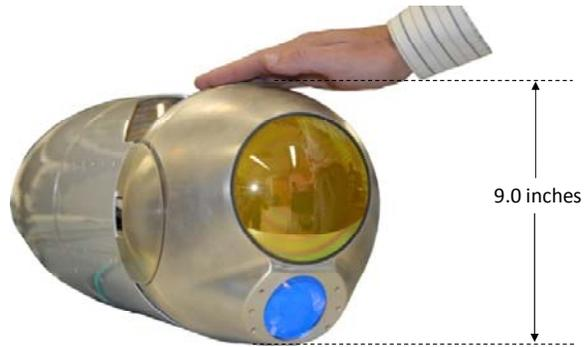
**Figure 2: Photograph of UAV instrument with LWIR dual-FOV telescope behind the yellow dome**
