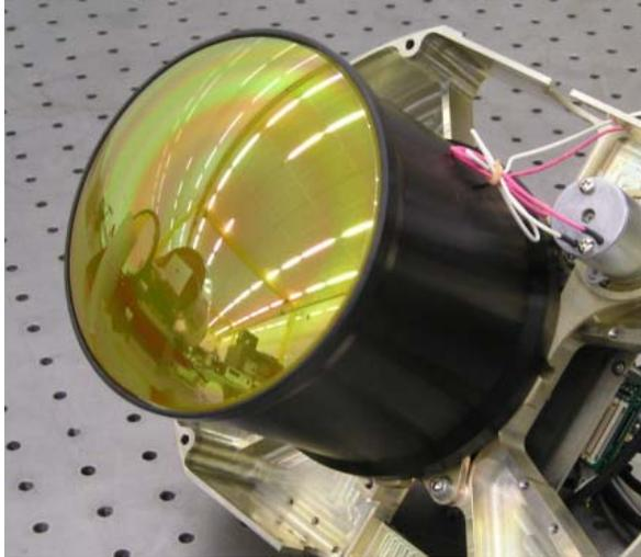
**Figure 1: Photograph of the compact, LWIR dual-FOV telescope. The compact nature of this design may be applied to any spectral band and application of interest.**
