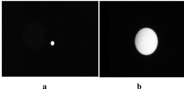
**Figure 10: Extended source images for the narrow FOV (a) and the wide FOV (b)**
