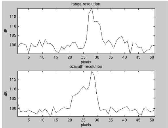
**Figure 7:** The range and azimuth response of target 1529A processed to a resolution of 0.6m per pixel.
