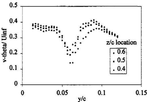
**Figure 2: Rotational Velocity at 6 degree angle of attack**
