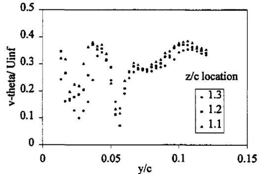
**Figure 3: Rotational Velocity at 8 degree angle of attack**
