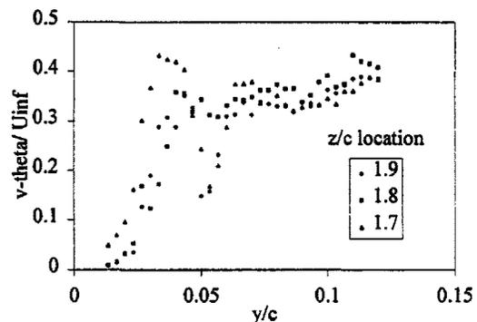
**Figure 4: Rotational Velocity at 6 degree angle of attack**
