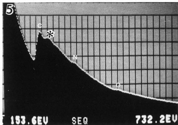
Figure 5. Electron energy loss spectrum obtained from a freeze-dried chromaffin granule. The various elemental K edges are indicated by their elemental symbol. The extra peak on the carbon edge (\*) results from plural scattering of the carbon K core-loss electrons. Vertical scale is 262,000 counts.
