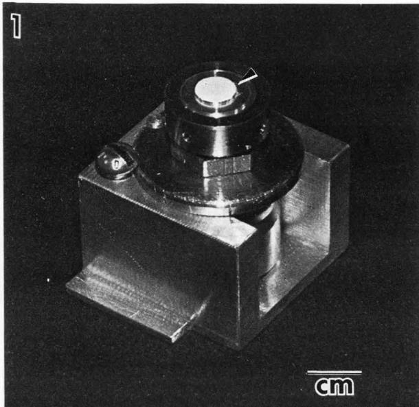
Figure 1. Modified Reichert specimen planchet holder and loading block assembly. The holder was remachined to mount a Balzers four position, freeze-etch specimen table to which the aluminum freezing disc (arrow) is held. The loading block is clamped in the knife position for specimen loading.
