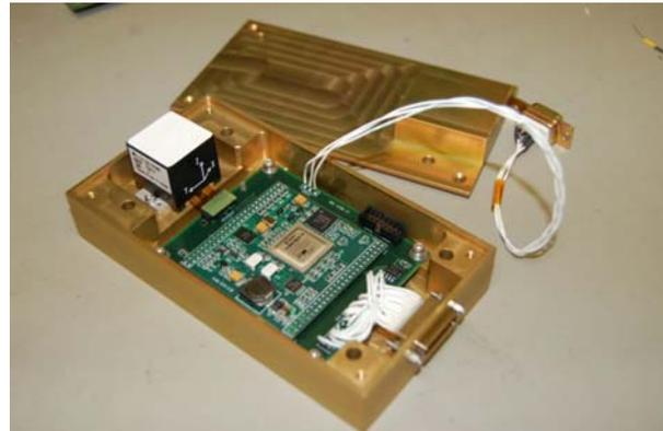
**Figure 5. Basic Elements of the PnP Sat IRU include a COTS MEMS IMU, and an ASIM for interfacing with the SPA protocol as well as providing processing for value-added software.**
