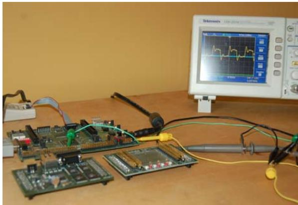
**Figure 4. Shown in a test configuration, the PnP MEMS IMU brassboard digital electronics for risk reduction of elements not available as COTS, as well as COTS implementation of those that are available for evaluation.**
