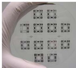
**Figure 2. MEMS IMU fabrication wafer with 12 dies, each with all the gyroscopes and accelerometers necessary to sense motion in six degrees-of-freedom.**
