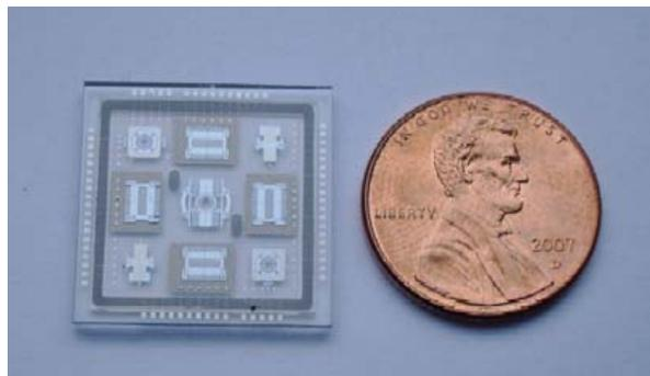
**Figure 1. MSSA MEMS IMU Sensor chip with 6-degrees of freedom based on 3 gyros and 6 accelerometers in a small package.**
