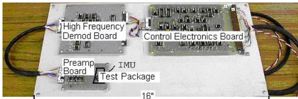
**Figure 3. The initial analog electronics for the gyro function is 16” long and 8” wide and includes the pre-amplifier board, the basic control electronics, and the high frequency demodulation board.**
