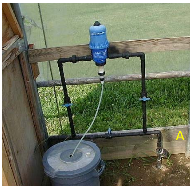
Image 1. A) Fertilizer injector used in high tunnels. B) Transplanted peppers growing under low tunnels on plastic mulch.
