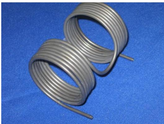
**Figure 2 The First Nitinol Coil (Dia ~2 inch)**
