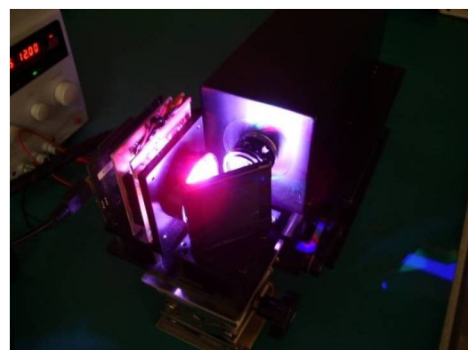
Figure 24: Overview of the spectral calibration by OCE for HSC-III spectrometer
