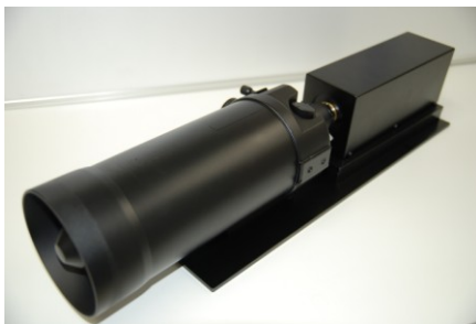
Figure 19: BBM of the HSC-III spectrometer equipped with CCD image sensor which has low-QE
