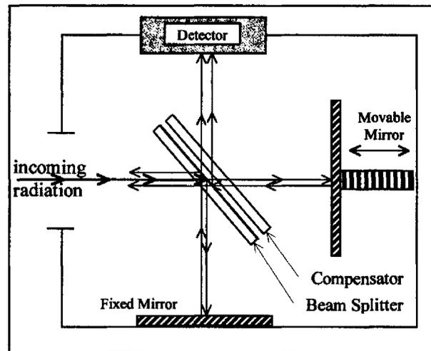
Figure 1. Michelson interferometer
