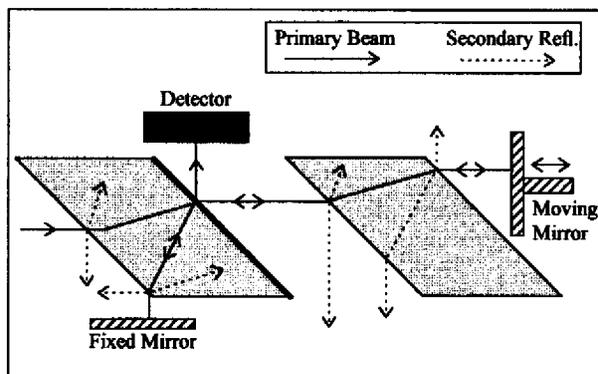
Figure 5. Dual Thick Slab with Widened Air Gap
