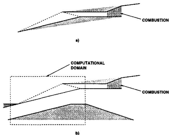
Figure 1: Schematic of (a) standard inlet and (b) thermal compression inlet.
