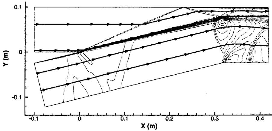
Figure 3: Streamlines and Horizontal-velocity contours for the thermal compression inlet, Mach 6 free stream.
