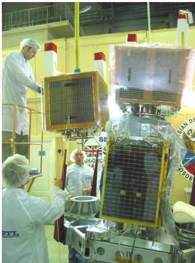
Figure 6. Accommodation of small satellites for a rideshare launch on the “Cosmos-3M” small launch vehicle
