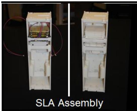
**Figure 1: Stereo Lithography Assembly of the SMDC-ONE Satellite**
