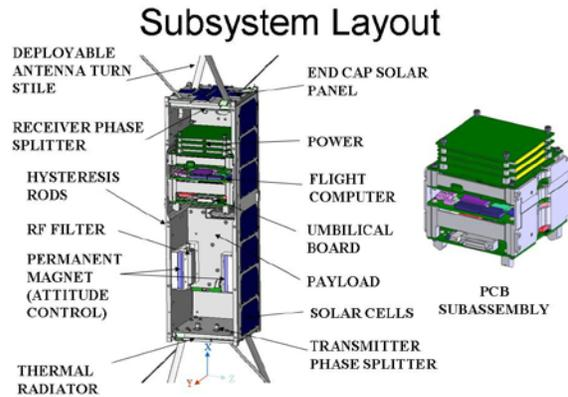
**Figure 2: SMDC-ONE Subsystem Layout**
