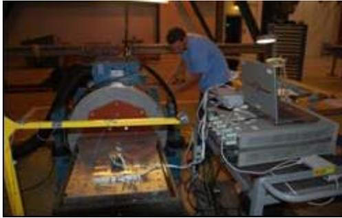
**Figure 4: Random Vibration Testing at Miltec's Iuka, MS Facility**
