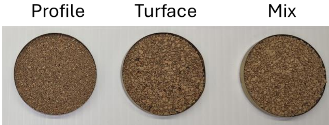
Figure 1. Calcined clay with three different particle size ranges: Profile (0.25-1 mm),
