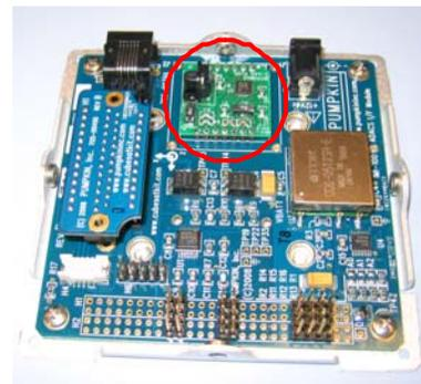
**Figure 3: MicroMag 3 Magnetometer (in red)**
