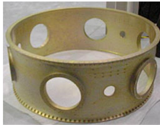
**Figure 1: EELV Secondary Payload Adapter (ESPA) with 15” Adapter Ring**
