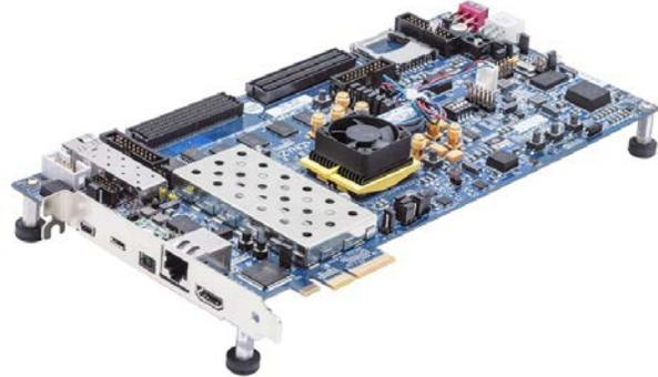
*Figure 4: Xilinx Zynq-7000 FPGA Development Board.*
