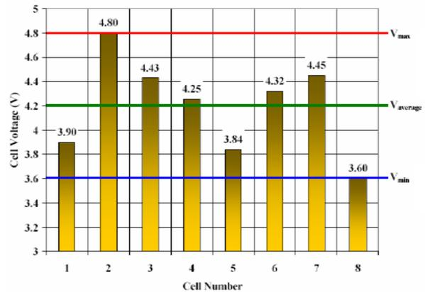
Figure 11: Indirect Overcharge
