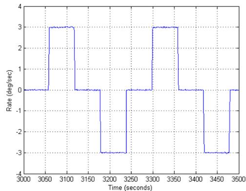
**Figure 10: IS Module Rate Output at +50degC with Temperature Compensation**
