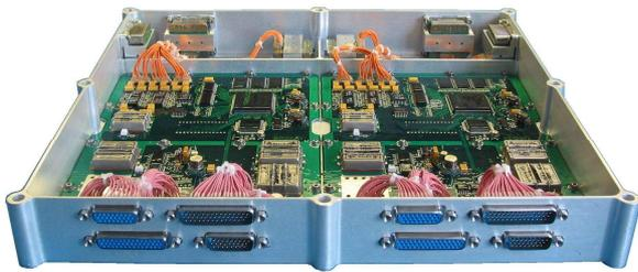
**Figure 8: Cold-Redundant Pair of Flight-Ready MIRaS-01 Modules**
