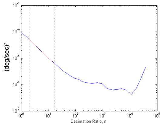
**Figure 9: Allan Variance Plot of 1Hz time-averaged output (raw sampling at 10Hz)**
