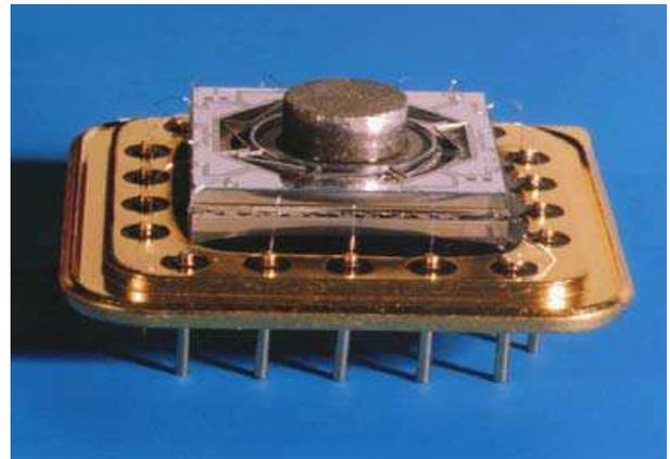
**Figure 2: Silicon Resonator**
