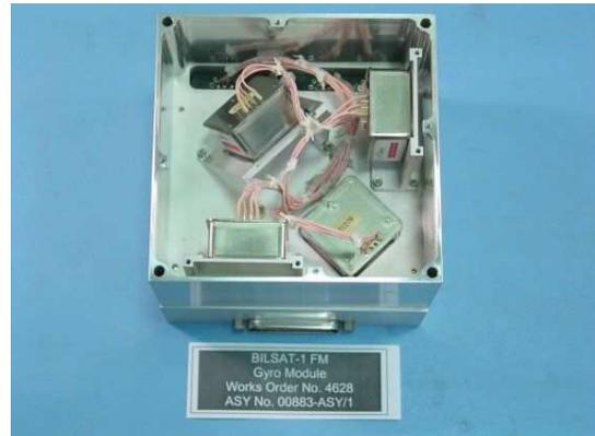
**Figure 6: Bilsat-1 Gyro Module**
