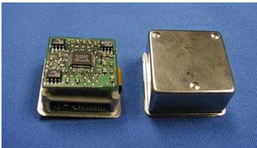
**Figure 5: Rate Sensor Control Board**
