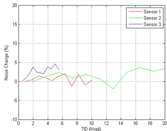
**Figure 12: Affect of TID on rate noise**
