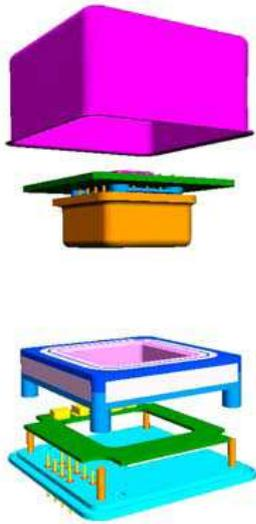
**Figure 4: Rate Sensor Construction**
