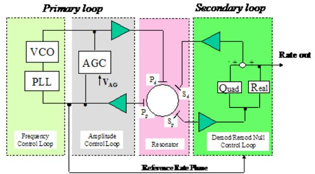
**Figure 1: Schematic of the rate sensor**
