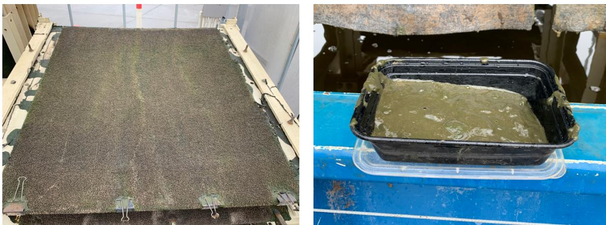
**Fig. 5.** Algae biofilm growth using the outdoor pilot-scale rotating algae biofilm reactor. The left image is before harvesting and the right image is after harvesting.
