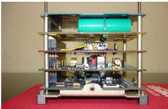
**Figure 7: The satellite has almost been fully integrated on the desktop chassis model in the lab and the final designs are being manufactured so that will go into the testing model currently being developed.**
