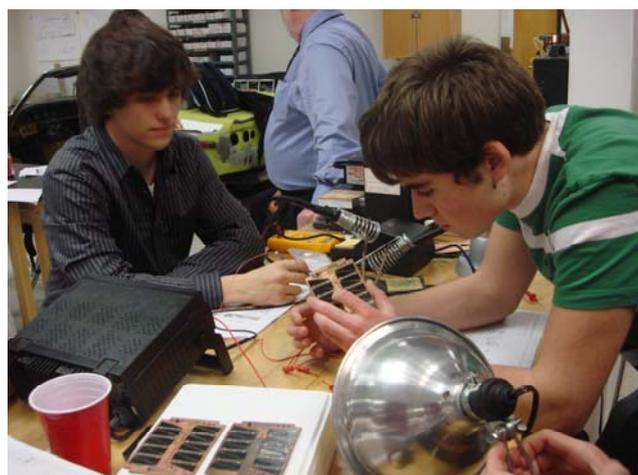
**Figure 6: Students learn many things in the midst of the development process, such as proper soldering techniques, the necessity of taking ESD precautions, and which methods do and do not work in manufacturing TJ<sup>3</sup>Sat's components.**
