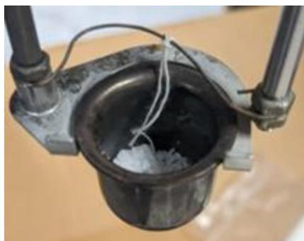
6. Close the bomb chamber and place in the calorimeter.
