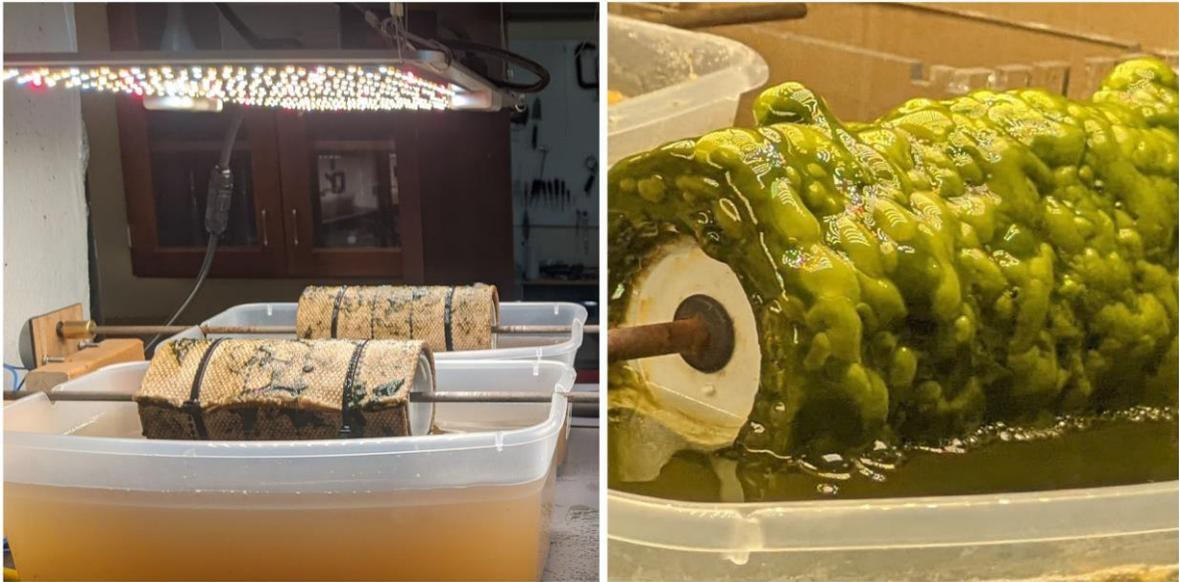
Figure 1. 5-L Rotating Algae Biofilm Reactors immediately after inoculation (left) and after biofilm formation (right).
