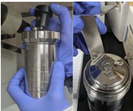
Image: pressure release tool (left) and cap release tool (right)
