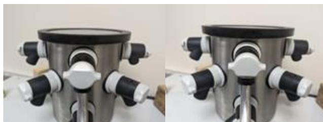
Image: open (right) and closed (left) sample valves
