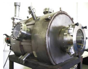
Figure 10: Thermal Vacuum Chamber
