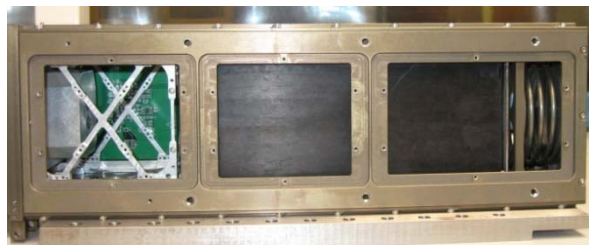
Figure 8: Poly CubeSat Launcher With Mass Models Inside
