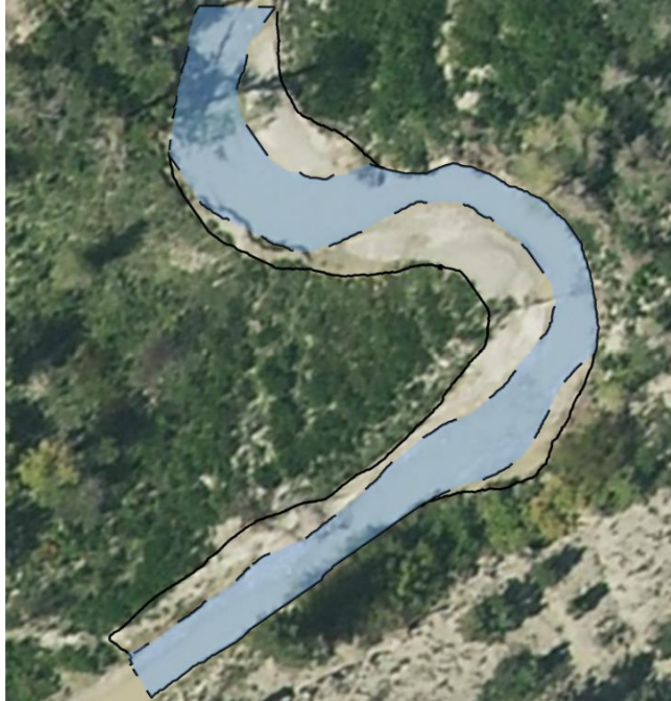
Figure 7. Screenshot of a bankfull indicators (point bars and vegetation) in a post-debris flow channel segment. The dashed line and light blue fill represent the visible water surface, and the solid line represents the approximate bankfull width.
