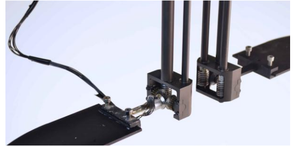
Figure 2: Flapping mechanism used for performing flapping kinematics with three independent rotational degrees of freedom including (pitch, sweep, and deviation).
