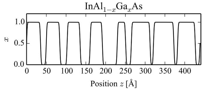
Fig. 1: A slice of the computational domain showing the layered structure of a single QCL period
