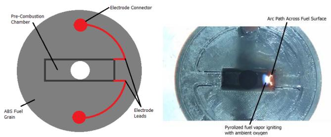
Fig. 1. Arc Ignitor Joule-Heating Concept Illustration and Demonstration.
