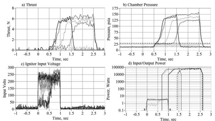
Fig. 2. Dual-shelf Ignitor, Co-Axial Injector Test Results.
