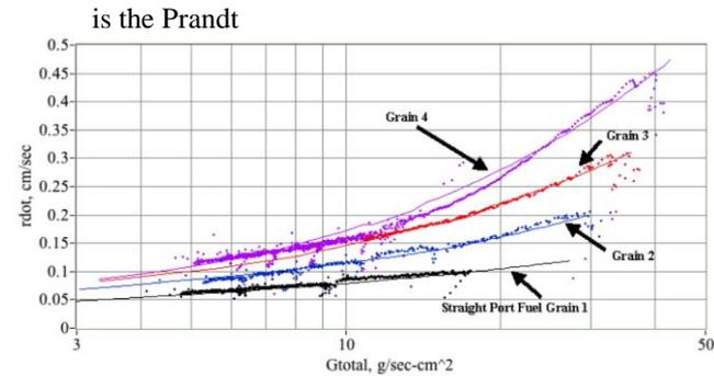
Fig. 6. Regression Rate Model Compared to Experimental Data
