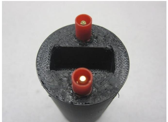
Fig. 9. Scaled-down fuel grain with integrated spark ignitor.
