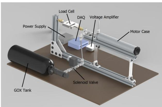
Fig. 7. CAD Drawing of Flight-Weight Integrated System
