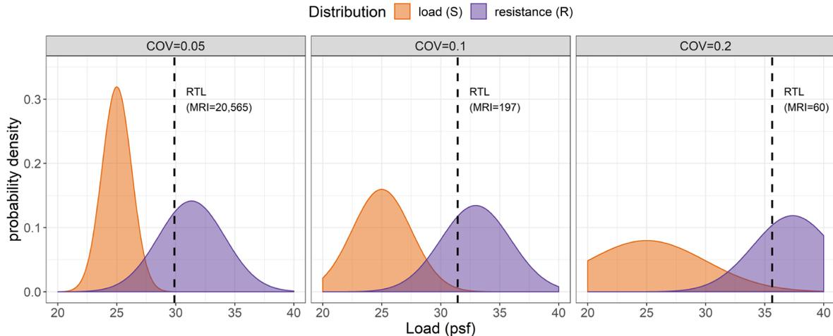
Figure 3. Illustration of the increase in reliability-targeted ground snow loads (RTL) due to increases in the coefficient of variation (COV) of the ground snow load distribution while the mean remains constant. These increases are associated with a reduction in the mean recurrence interval (MRI) of the nominal ground snow load, as indicated by the increasing area under the orange curve to the right of the dashed line.
