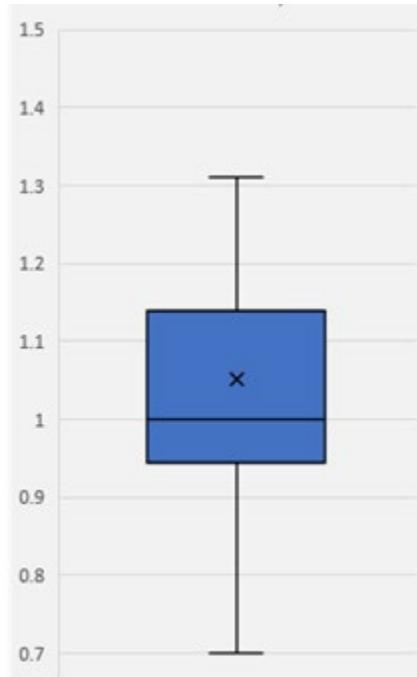
Figure 2. Box plot of the ratio of proposed factored loads to previous factored loads. Average ratio: 1.05, Standard Deviation: 0.21.
