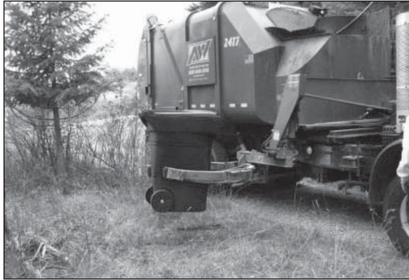
Figure 1. Driver picking up the automated Kodiak container ( Photo courtesy of G. Barce ).
