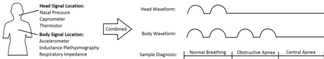
**Figure 3:** Method for combining head and body signals in a way that differentially identifies central and obstructive apnea. When there are no breaths in either signal, central apnea is marked. If there are breaths in the body waveform and no breaths in the head waveform, obstructive apnea is marked.
