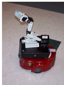
Fig. 2.7: Bioloid arm platform.
