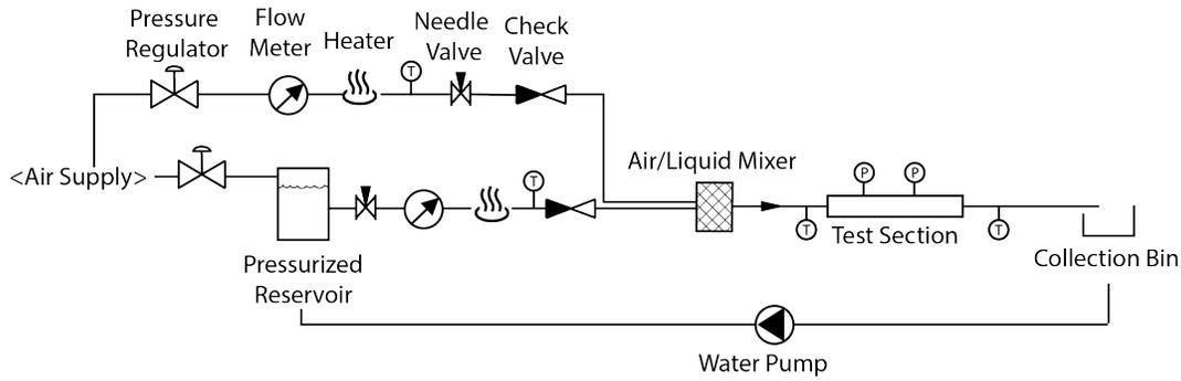
Fig. 3. Schematic of the two-phase flow loop.
