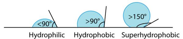
Fig. 1. The solid-liquid contact angle determines the hydrophobicity of a surface. Hydrophilic surfaces have a contact angle less than  $90^\circ$ , while hydrophobic surfaces have contact angles greater than  $90^\circ$ . Superhydrophobic surfaces have a solid-liquid contact angle of greater than  $150^\circ$ .
