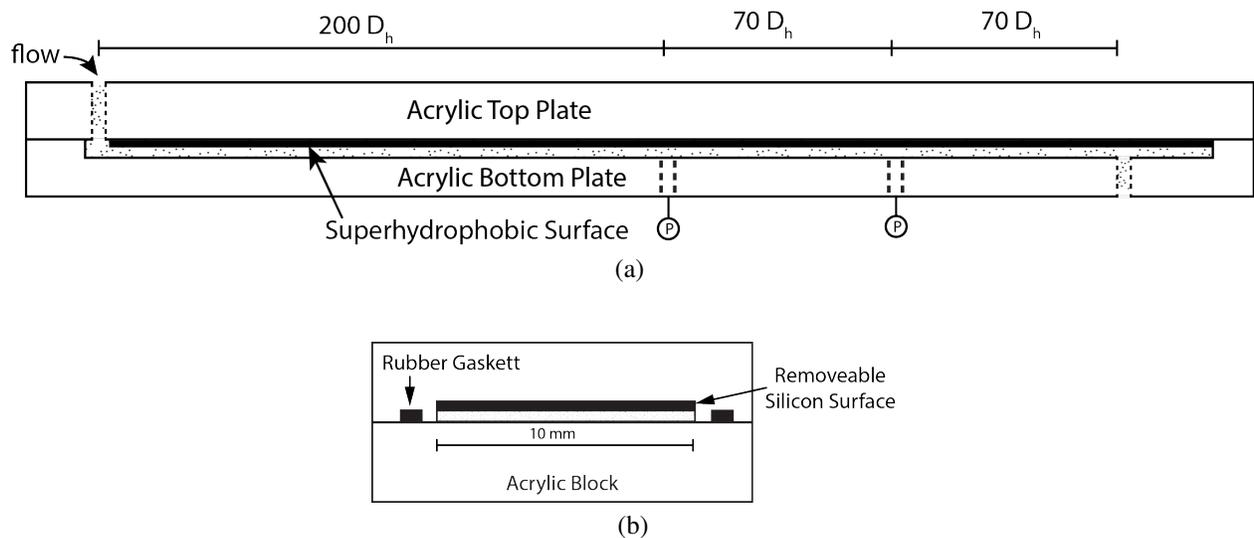
Fig. 4. The test section (a) has a hydraulic diameter of about  $700 \mu\text{m}$ , a height of  $300 \mu\text{m}$ , and a width to height ratio of 30. A cross-sectional view of the channel is shown in (b).
